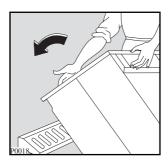
Carefully remove the polyethylene bags located at the base of the machine by pulling them toward the centre of the machine.
